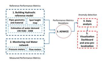
Figure 1. Model-based FDD methodology.
