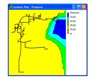
Figure 6. Output in term of pressure for the WDS model with leakage scenario SP8.
