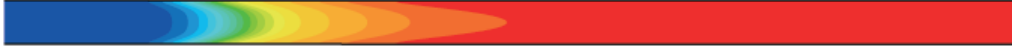
Fig. 3. Contours of mole fraction of C_{(s)} at 900 °C and 20 mbar partial pressure of acetylene
