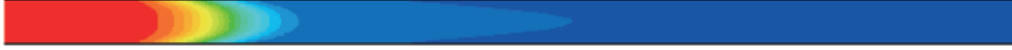
Fig. 2. Contours of mole fraction of C_2H_2 at 900 °C and 20 mbar partial pressure of acetylene
