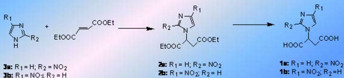
**Scheme 1.** Addition of nitroimidazoles to diethyl fumarate under different conditions
