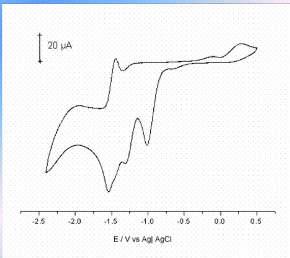
**Figure 6.** Cyclic voltammogram of **1b** in anhydrous DMF + 0,1M  $BF_4(n-Bu)_4NH_4$ . Sweep rate  $100$  mV s<sup>-1</sup>
