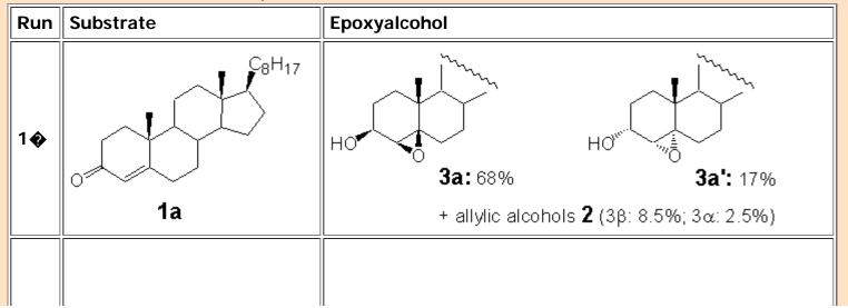
Table. One-Pot Reduction  $\Rightarrow$  Epoxidation Reaction of a,b-Unsaturated Ketones with DIBAH and t-BuOOH
