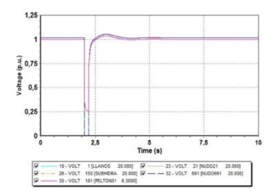
Voltage dips in isolated systems are very deep and their area of propagation is very wide-spread.
