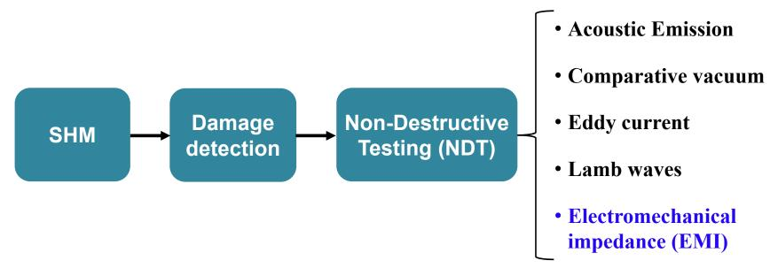
The electromechanical impedance (EMI) method stands out from the other methods by its simplicity and by using low-cost, lightweight and small piezoelectric transducers
