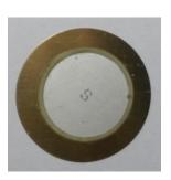
Piezoelectric diaphragm – "Buzzer"
