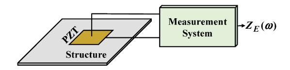
$$Z_{E}(\omega) = \frac{1}{j\omega C_{0}} ||jZ_{T}\left(\frac{s_{11}}{d_{31}\ell}\right)^{2} \left[\frac{1}{2} \tan\left(\frac{k\ell}{2}\right) - \frac{1}{\sin(k\ell)} + \frac{Z_{S}}{j2Z_{T}}\right]$$
