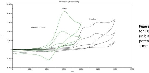
**Figure :** Selected cyclic voltammograms at a Cv electrode for ligand **1** (in green) and rhenium complex  $[Re(CO)_3(1)]$  (in black), in MeCN,  $[Bu_4NCIO_4] = 0.1 \text{ mol.L}^{-1}$  at different potential scan rates 0.1, 1 and 4 V/s; analyte concentration 1 mmol.L<sup>-1</sup>.
