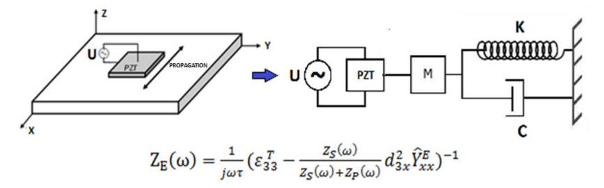
According to equation, any variation in the mechanical impedance " $Z_S(\omega)$ " of the structure caused by damage involves a corresponding variation in the electrical impedance " $Z_E(\omega)$ " of the transducer
