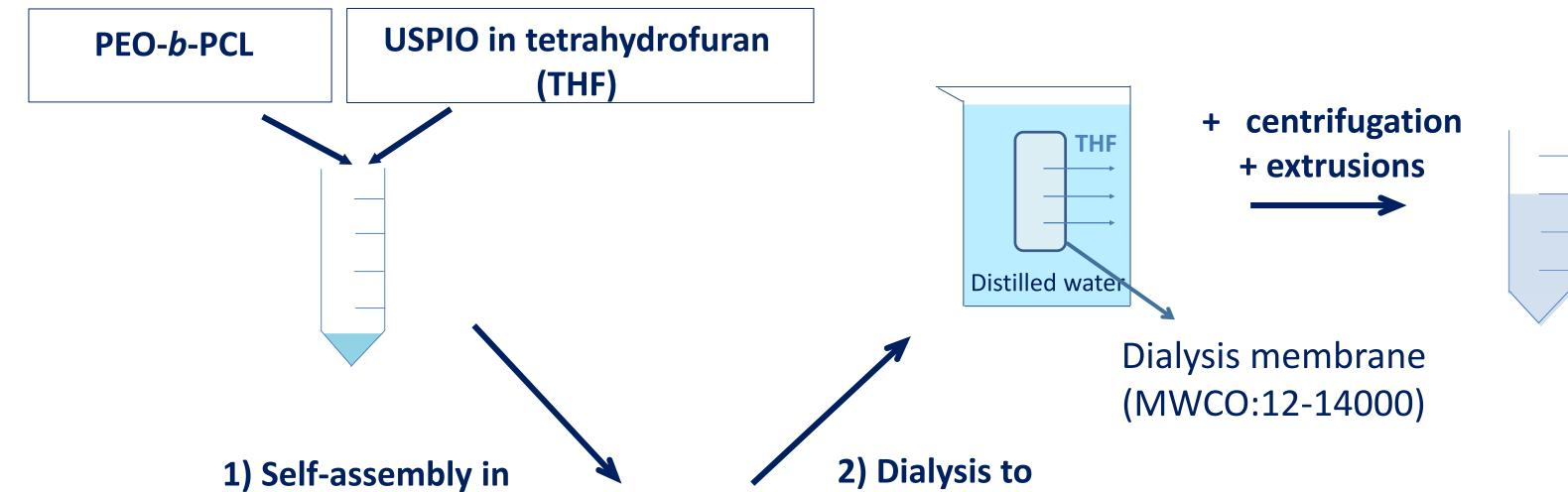
USPIO (magnetic core size of 4.2 nm and 7.5 nm) were produced by thermal decomposition of iron(III) acetylacetonate in the presence of surfactants in an organic solvent at high temperature (>200°C).
