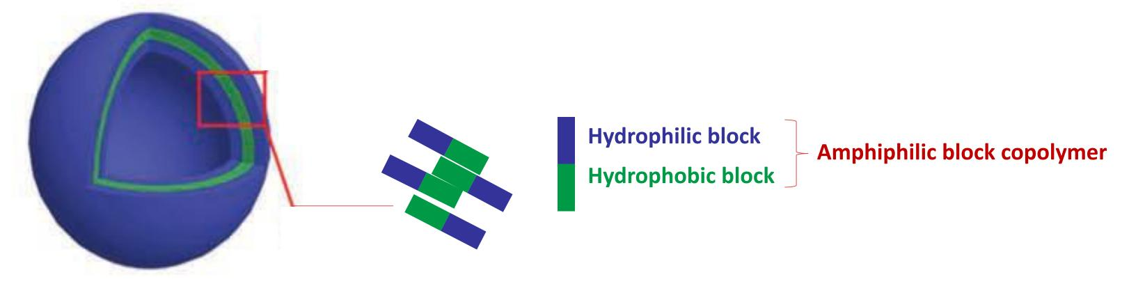
*Figure 1.* Schematic representation of a polymersome
