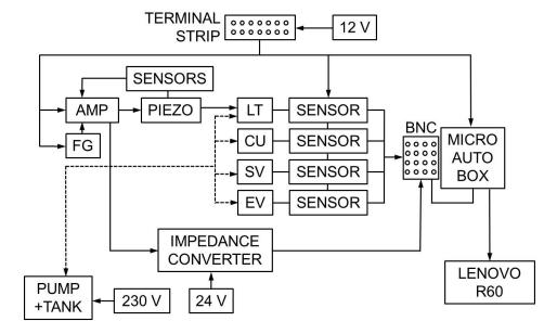
Figure 1. Block diagram of the indirectly controlled FVVT system.
