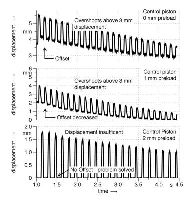
Figure 6. Control piston displacement in dependency of chosen return spring preload.
