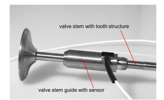
Figure 3. Sensitec GLM700 FVVT valve travel sensor application.
