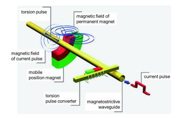
Figure 4. Principle of magnetostrictive displacement measurement.
