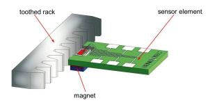
Figure 2. Sensitec GLM7xxASB-Ax sensor composition [1].
