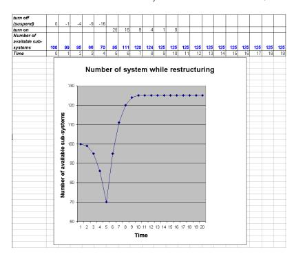
Figure 1. Changes in the number of available subsystems during an adaptation process.) After a successful restructuring (Time=5) the sub-systems' activity is re-enabled. This (re-)activation is spreading like an epidemic but in a reverse order. The parent system now includes the newly connected sub-system (in our case additional 25)
