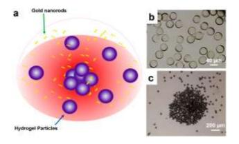
Figure 1. Principle of light assembly of microparticles through plasmonic nanoparticles (gold nanorods (GNRs))
