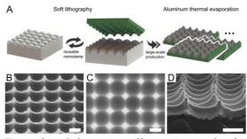
illustration 2. Schematic ofthe Fig. procedure offabrication NPA Alnanostructures by ESL and subsequent Al deposition. The elastic nanostamp is molded from a NPA fabricated through EBL and electrochemical etching, and used repeatedly for high throughput of NPA substrates composed of transparent polymer and Al nanostructures.
