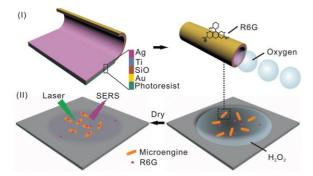
Fig.1 Schematic illustrations: (I) the fabrication process of Au/SiO/Ti/Ag tubular microengines by employing rolled-up nanotechnology and (II) the microengines adsorbed analyte molecules (R6G) in the fluids for SERS measurement..
