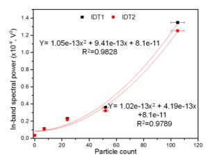
Fig.4 Experimental results for the SAW-PA sensing of the particles. Power spectral density (9-11 MHz) for various particle concentrations is calculated at the two sensing IDTs. The spectral power exhibits second order response with particle concentration.
