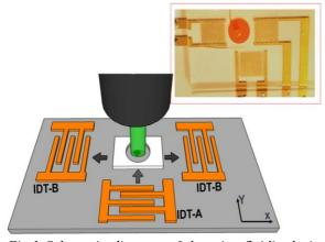
Fig.1 Schematic diagram of the microfluidic device with the concentrating (IDT-A) and sensing (IDT-B) interdigital transducers (IDT). A pulsed laser irradiates on the particle inside the reservoir to generate a SAW. Inset shows the photograph of the fabricated SAW device.
