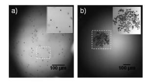
*Fig. 3 Particle-laden cavity before (a) and after (b) SAW exposure for 50 sec.*
