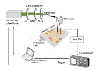
Fig.2 Schematic of the experimental setup used for SAW-PA detection of microparticles inside a microfluidic reservoir.
