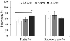
Fig.4 Effect of square light patterns rotating rate (3.5, 7, and 14 RPM) on the CTC clusters isolation purity (%) and recovery rate (%) at the side microchannel (\*p<0.05, ANOVA).
