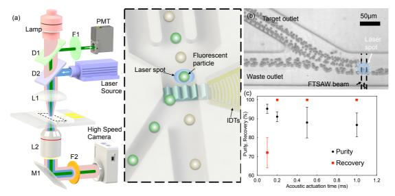
Fig. 1. (a) Schematic illustration of our acoustic fluorescence activated cell sorting (FACS) system. (b) Time-lapsed photos of the particles sorting process based on their fluorescent label. (c) Correlation between the sorting performance (purity and recovery) and the acoustic actuation time of each sorting event.
