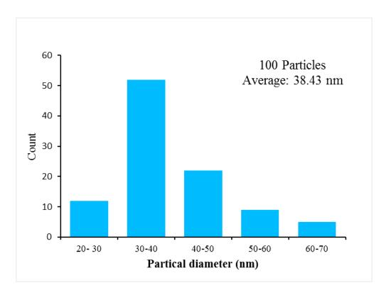
Fig.3. Distribution diagram of particles size of Fe<sub>3</sub>O<sub>4</sub>
