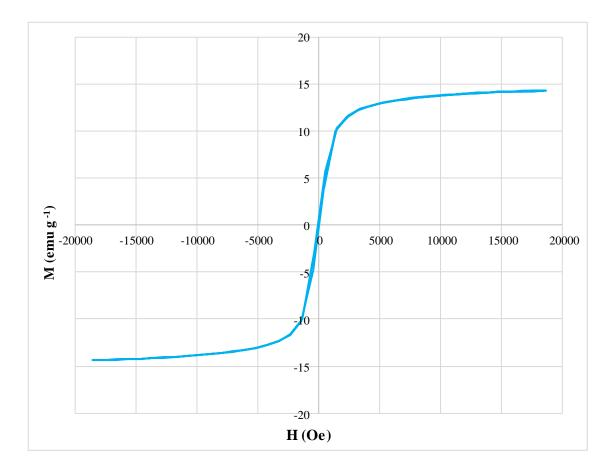
Fig. 4. VSM curve of gelatin/Fe<sub>3</sub>O<sub>4</sub>/ ethylene glycol hydrocarbon gel nanocomposite
