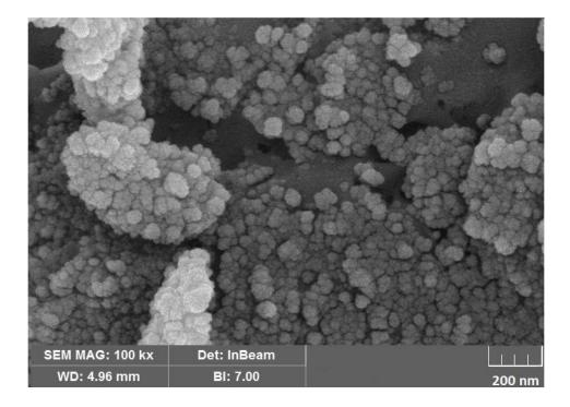
Fig. 2. SEM images of gelatin/Fe<sub>3</sub>O<sub>4</sub>/ ethylene glycol hydrocarbon gel nanocomposite
