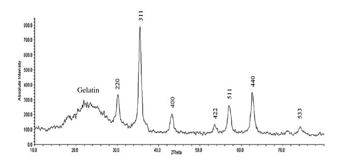
Fig. 1. XRD patterns of gelatin/Fe<sub>3</sub>O<sub>4</sub>/ ethylene glycol hydrocarbon gel nanocomposite
