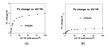
**Figure 3.** The dependence of the V<sup>T</sup> increase on UV irradiation TD for an F-SOHOS capacitor (**a**) under gate PVS 20 V; (**b**) under gate PVS 10 V.
