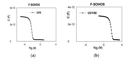
**Figure 2.** This CG-VG curve for an F-SOHOS capacitor device (**a**) before UV irradiation; (**b**) after UV TD 100 mW·sec/cm<sup>2</sup> irradiation.
