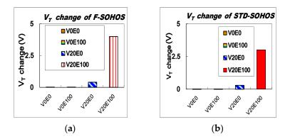
**Figure 4.** (a) The V $_{T}$  change of F-SOHOS capacitor devices after various UV irradiation; (b) The V $_{T}$  change of STD-SOHOS capacitor devices after various UV irradiation.
