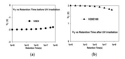
**Figure 5.** The VT vs. retention time for an F-SOHOS device: (a) before UV irradiation, and (b) after UV TD 100 mW·sec/cm<sup>2</sup> irradiation under gate PVS 20 V.
