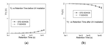
**Figure 6.** The comparison of V<sub>T</sub> vs. retention time for F-SOHOS and STD-SOHOS devices: (a) before UV irradiation; (b) after UV TD 100 mW·sec/cm<sup>2</sup> irradiation under gate PVS 20 V.
