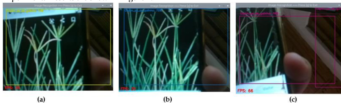
Figure 4. Real Time Weed Detection Results: (a) Capim pé de Galinha weed detection with float32 quantization, (b) Capim pé de Galinha weed detection with float16 quantization (c) Capim pé de Galinha weed detection with int8 quantization. (Source: Designed by the authors).
