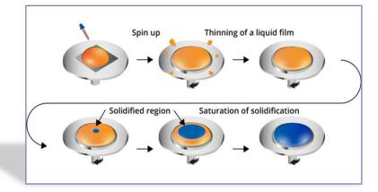
Thin films from polymer of 24% acetal content were deposited with approximate thickness of 80 nm on PET flexible substrate by the method of spin coating using 0.250 ml of 1 wt% solution of polymers in 80:20 volume ratio of methanol-to-water solvent.
