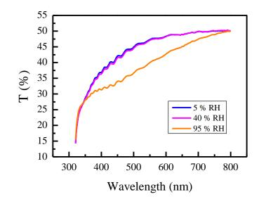
Transmittance spectra T for humidity levels of 5 %, 40 % and 95 % RH of sample after each set of bends were measured.
