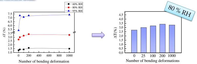
Transmittance change  $\Delta T$  is calculated for each set of bends and for three different humidity levels – 60 %, 80 % and 95 % RH.
