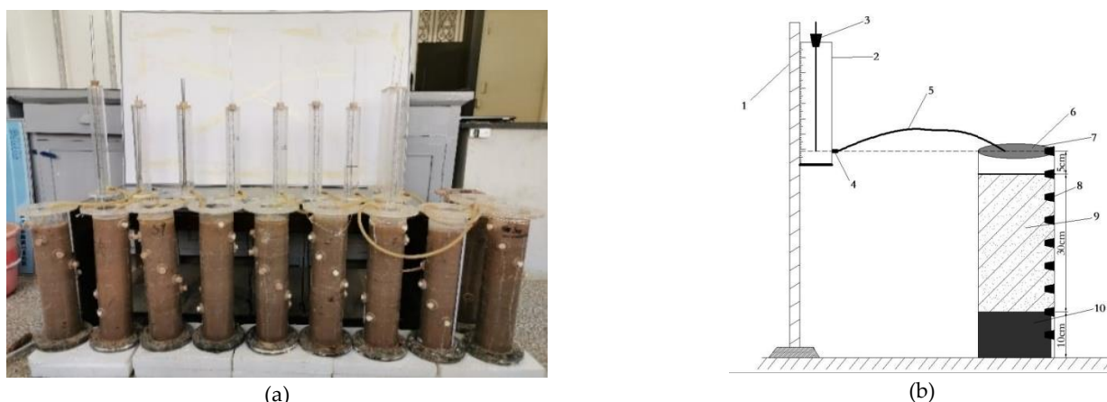
Figure 1. View of the laboratory experiment to assess the infiltration and salt leaching. (a) disposal of soil columns; (b) Column scheme; Legend: 1. bracket, 2. Marten site bottle, 3. level index, 4. valve, 5. hose, 6. plastic film, 7. column top, 8. sampling hole, 9. soil sample with added sand, 10. original soil.
