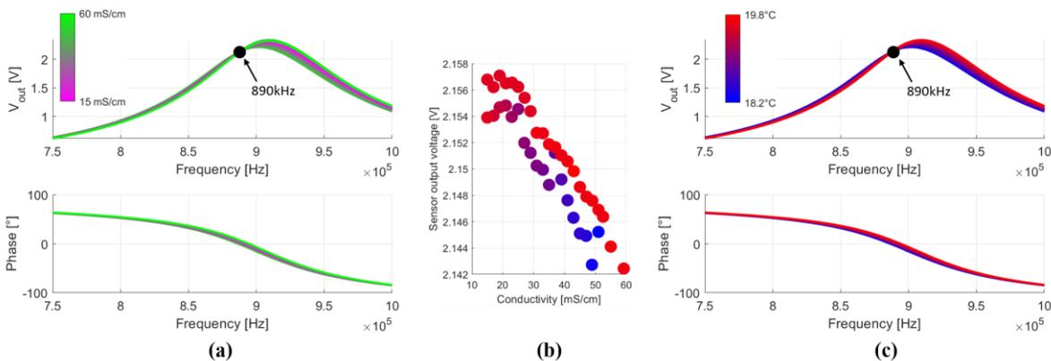
Figure 3: Frequency spectrum for the sensor output voltage coloured for (a) conductivity and (c) temperature. In (b): Output voltage at 890kHz plotted over conductivity with temperature colour grading.
