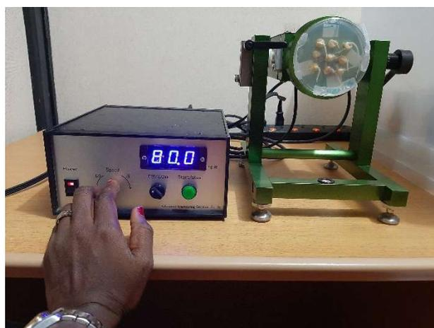
**Figure 1.** 2-D Clinostat at the Microgravity Simulations Laboratory, National Space Research and Development Agency (NASRDA), Abuja, Nigeria.
