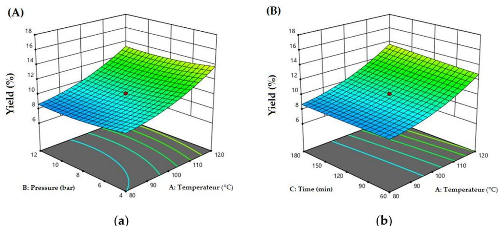
**Figure 1.** Response surface plot demonstrating the effect of (a) temperature and pressure and (b) temperature and extraction time on %yield of polysaccharides.
