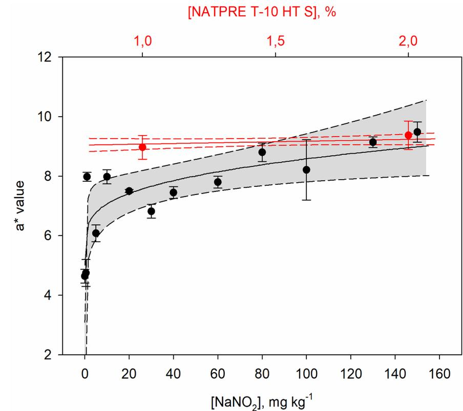
Figure 1. Influence of the presence of both sodium nitrite and NATPRE T-10 HT S on the color of cooked ham samples
