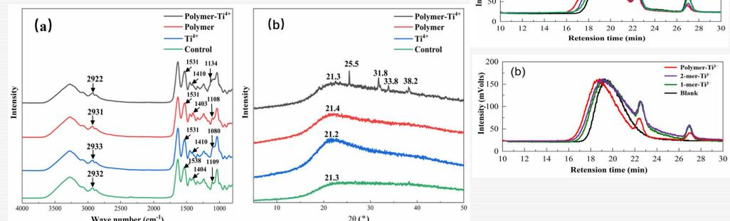
New peaks were identified after crosslinked by PA-Ti<sup>4+</sup>, represent the chelating reaction between PA and Ti<sup>4+</sup> within gelatin film. a gradually increasing gelatin molecular weight after crosslinking treatment. Furthermore, the molecular weight of the gelatin was also affected by the type of the crosslinker, the higher the PD of the PA, the higher the gelatin molecular weight were observed.
