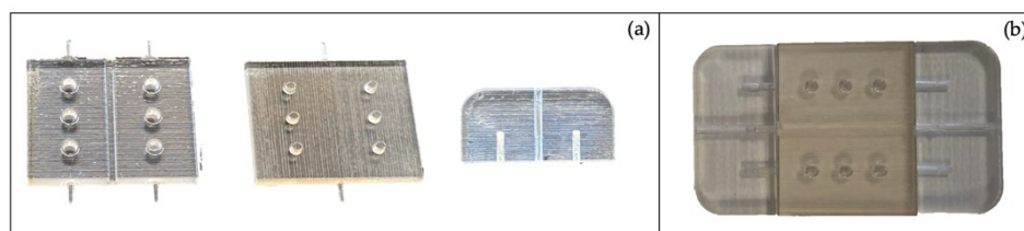
Figure 2. a) SPR sensor’s 3D printed disassembled parts. b) Assembled SPR sensor.
