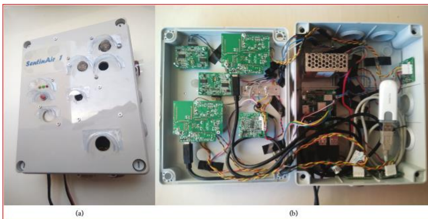
Fig. 2. The figure shows (a) the complete set-up of the low-cost sensor, and (b) the inlet of the sensor showing the power charger and other parts
