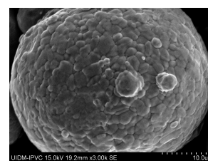
Figure 3. SEM images at 3000× magnification of Tool Steel 1.2709-A LMF (TRUMPF) powder particle.
