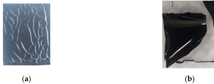
Figure 2. Effect of the weight ratios of PVA-PEO blends on the physical properties of the films: (a) 3.5:1; (b) 1:3.5.
