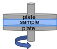
Parallel plates, 25 mm in diameter, and gap
