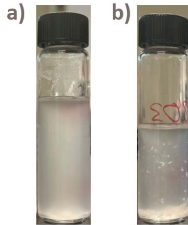
5 6 Figure 5. Images showing a dispersion of liposomes loaded with hyaluronic acid at physiological 7 pH (a) and a dispersion of liposomes and aggregate hydrogel particles at pH 2.03 (b).
