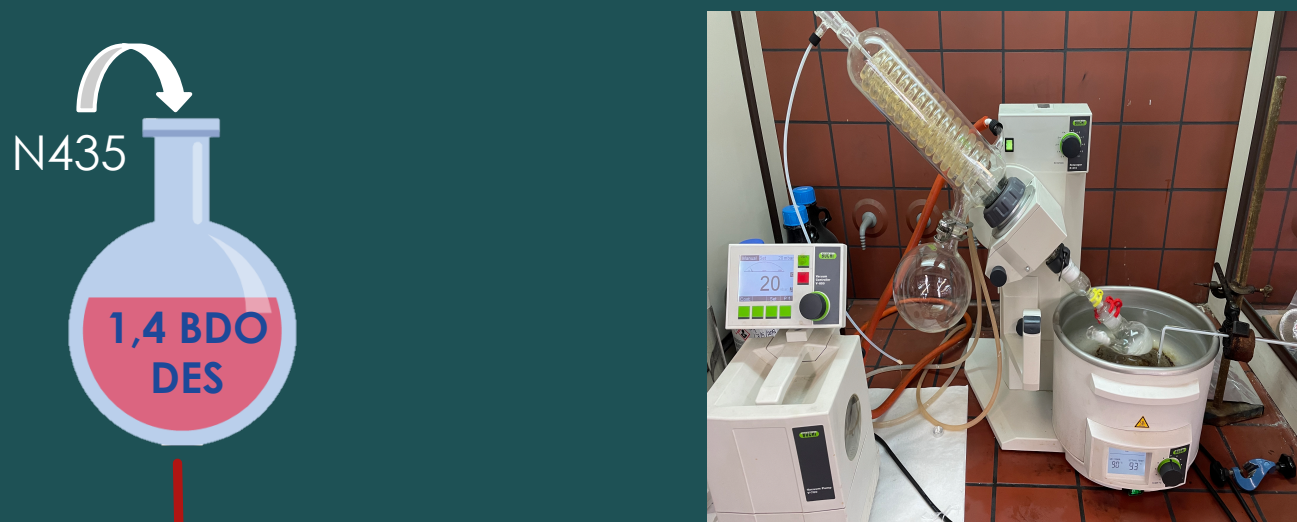
Figure 1. Apparatus for the production of PBS oligomers
