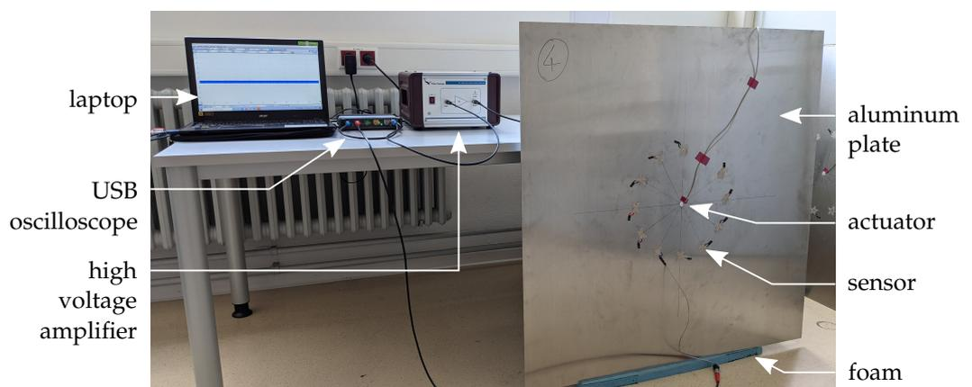
**Figure 2.** Test setup to determine the peak-to-peak voltage of the sensors under GUW excitation
