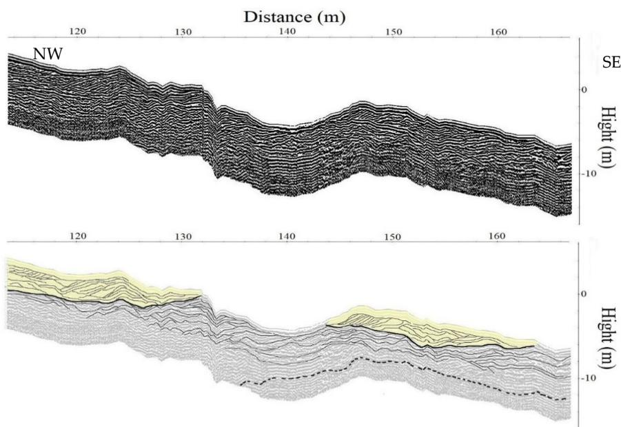
**Figure 4.** Part of the radargram corresponding to the beach-crest transect and its corresponding interpretation.
