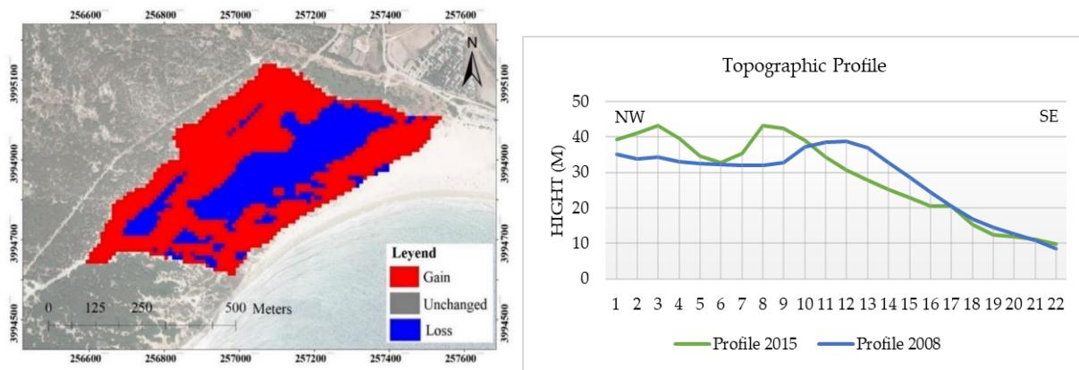
**Figure 2.** **Left:** Volumetric variation representation of the Valdevaquerros dune, showing loss and gain zones (blue and red) between 2008 and 2015. **Right:** Topographic Profile of the Valdevaquerros dune for 2008 and 2015.
