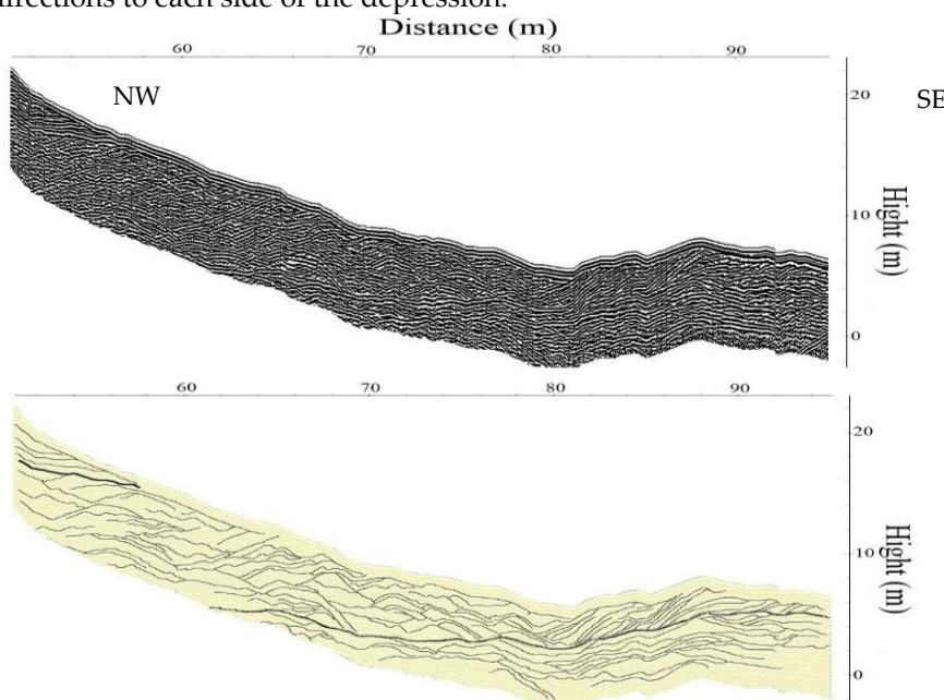
**Figure 3.** Part of the radargram corresponding to the beach-crest transect and its corresponding interpretation.
