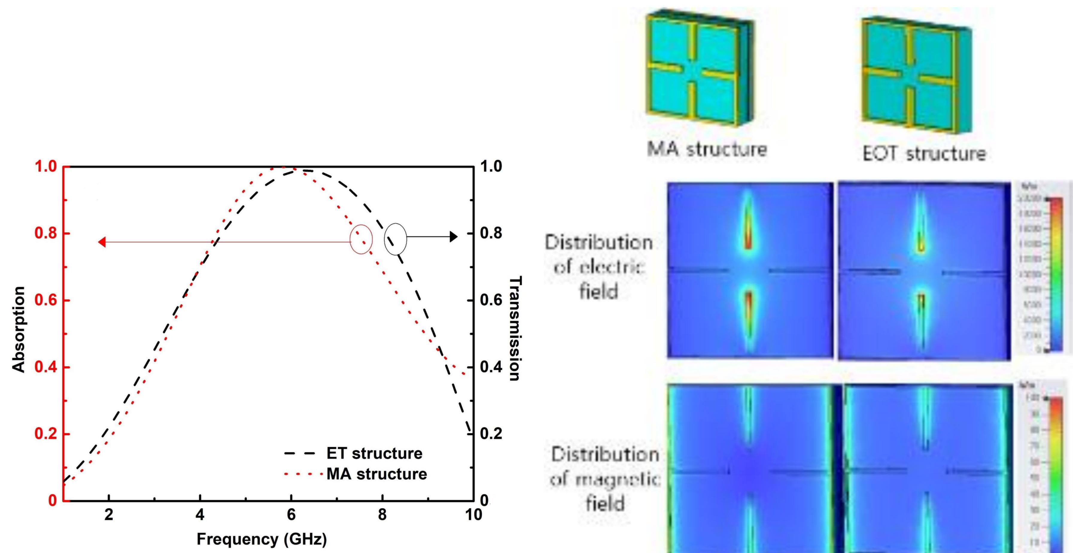
Two spectra very close but the spectrum of transmission broader than that of absorption. The localized electric and magnetic fields on the surface of MA structure seem to be stronger than that those of EOT one.
