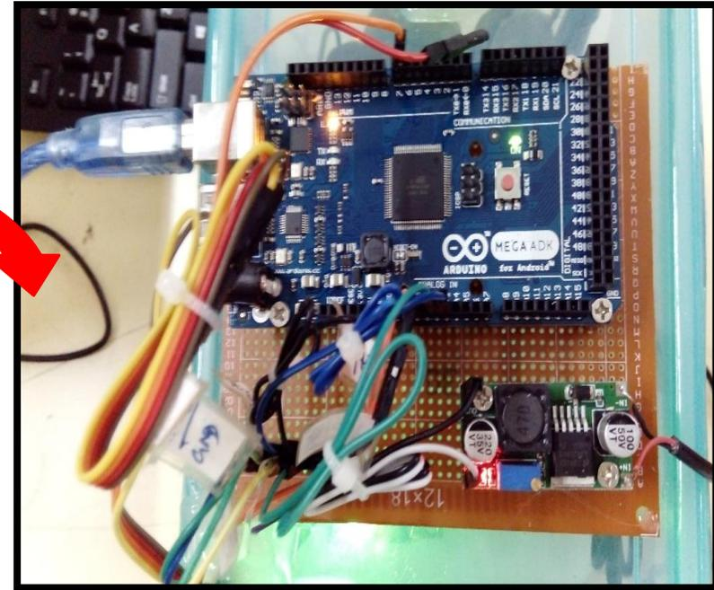
Arduino MEGA 2560 microcontroller board connected with sensors & attached to the top surface of the fermenter.
