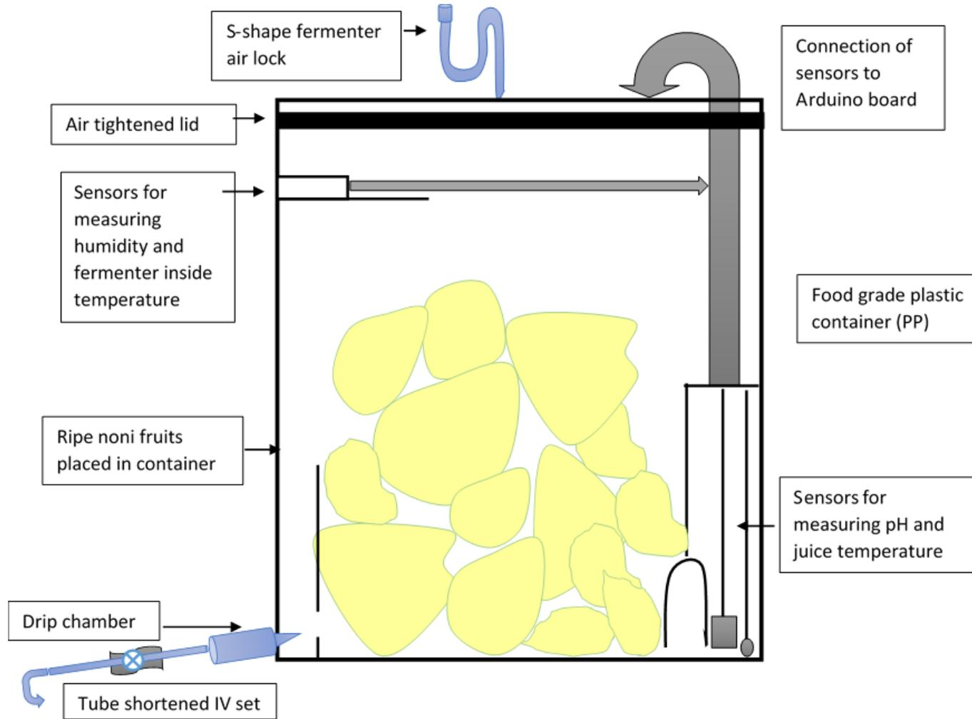
**Schematic Diagram of the Fermenter**
