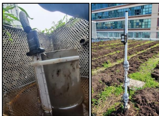
Figure 5. Sensor fixed to the drain ( left ) and node mounted on the pole ( right ).
