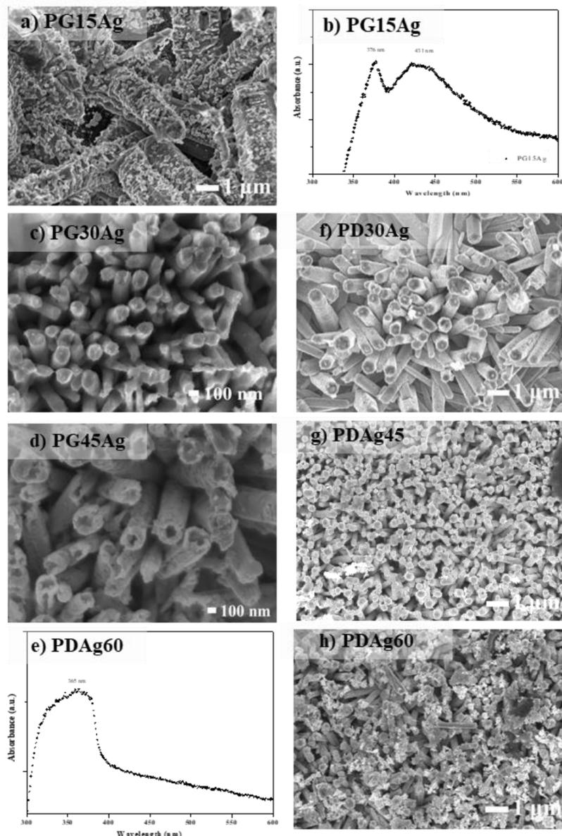
Figure 1. SEM images of photogrown (a,c,d) and photodecorated (f, g,h) Ag-NP@ZnO-NC substrates. Absorbance spectra of PG15Ag (b) and PDAg60 (e) samples.
