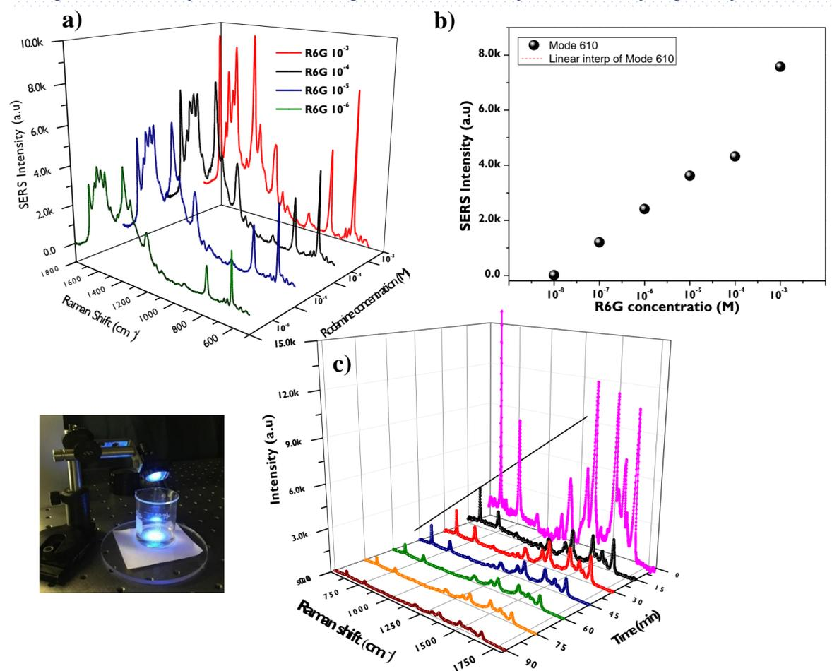
Figure 3. a) Raman spectra of the SERS PG30Ag/R6G substrate at different R6G concentrations b) SERS intensity of the 610 mode at different R6G concentrations c) Cleaning of the substrate by UV irradiation at different times.
