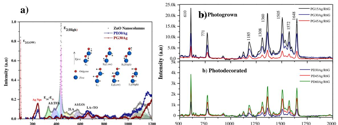
Figure 2. a) Raman spectra of ZnO NCs and Ag-NP@ZnO-NC substrates photodecorated (PD30Ag) and photogrown (PG30Ag) during 30 min. b) Raman spectra of  $10^{-3}$  M R6G in Ag-NP@ZnO-NC substrates photodecorated and photogrown deposition.
