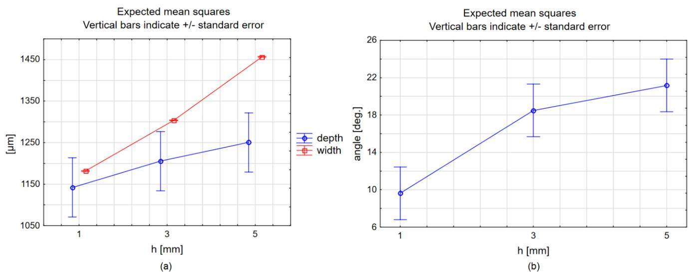
**Figure 2.** (a) Relation between abrasive mass flow rate and grooves' depth and top kerf width. (b) relation between abrasive mass flow rate and kerf taper angle.
