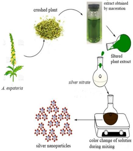
*Figure 1.* Graphic representation of the green synthesis of silver nanoparticles
