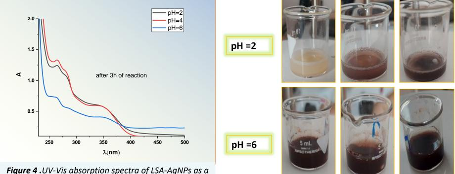
**igure 4**.UV-Vis absorption spectra of LSA-AgNPs as function of *npH* value
