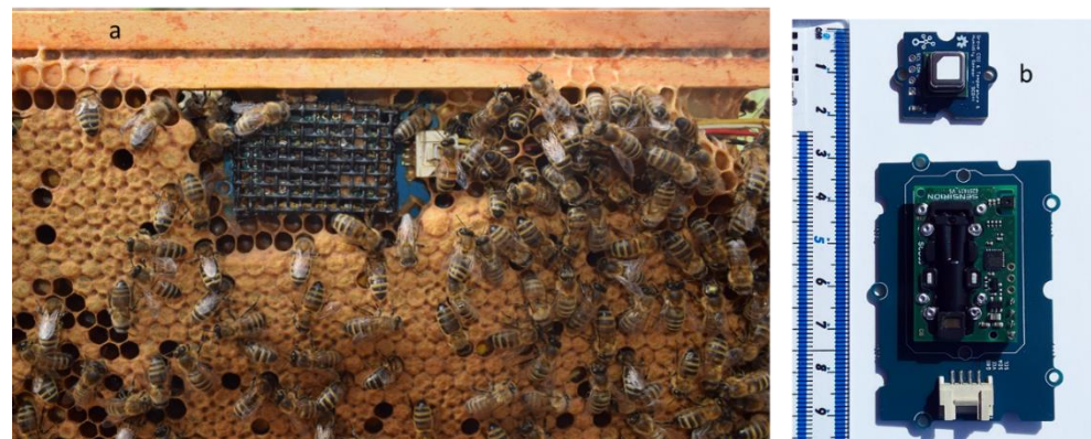
Figure 1. (a) SCD30 installed in brood box frame showing propolis coating on the protective mesh. (b) SCD30 (lower) and SCD41 (upper) sensors with rule to show relative sizes of the two devices.
