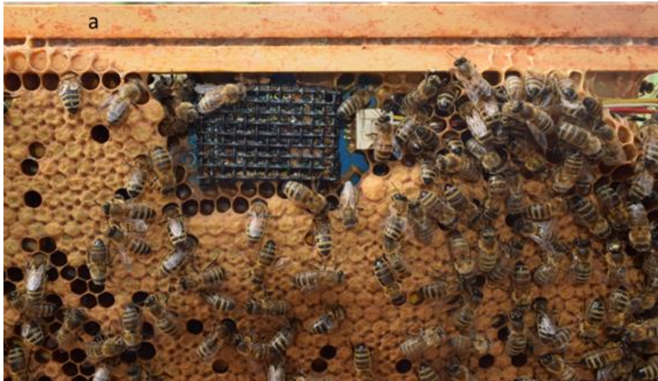
(a) SCD30 installed in brood box frame showing propolis coating on the protective mesh.
