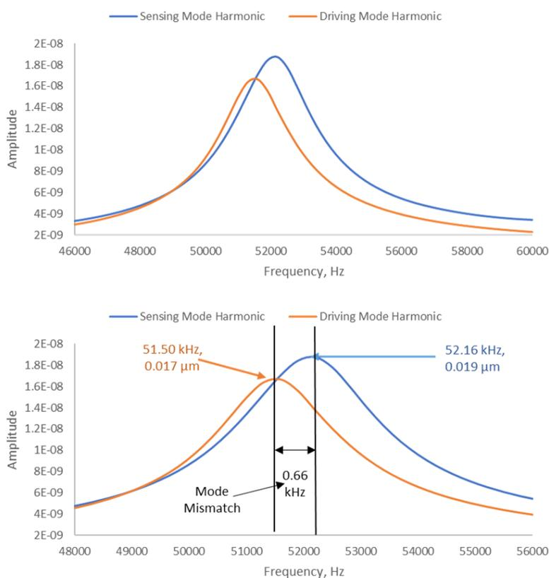
Figure 6. A harmonic response for the amplitude-frequency response.
