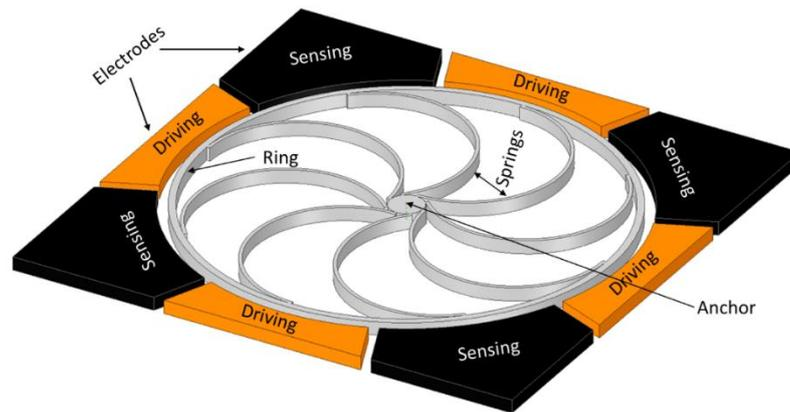
**Figure 2.** A schematic view of vibratory ring gyroscope.
