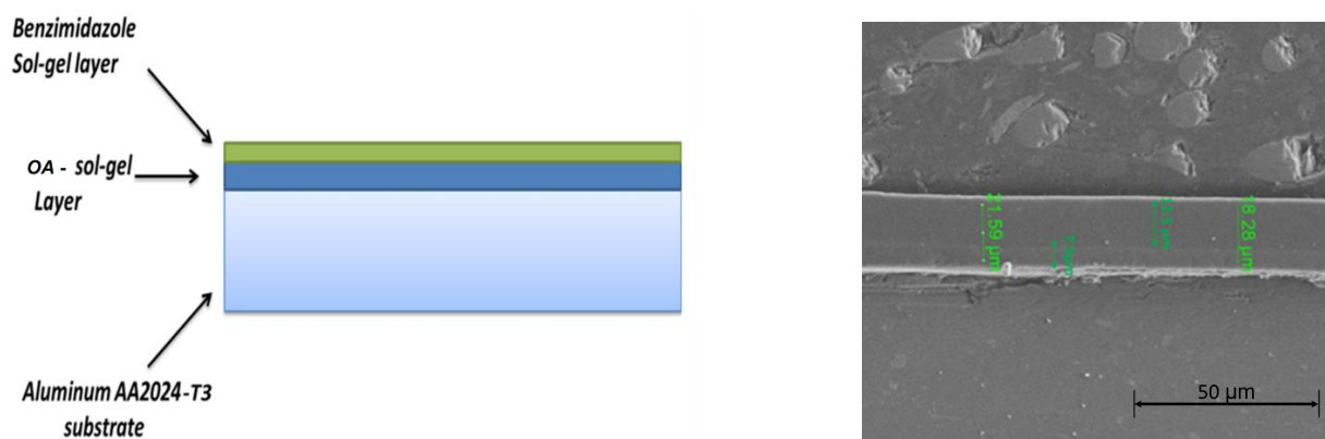
Figure 2. schematic of the double layer sol-gel coating system of BZI and OA, and SEM cross-section image of BZI-OA-SHX sol-gel coating system.
