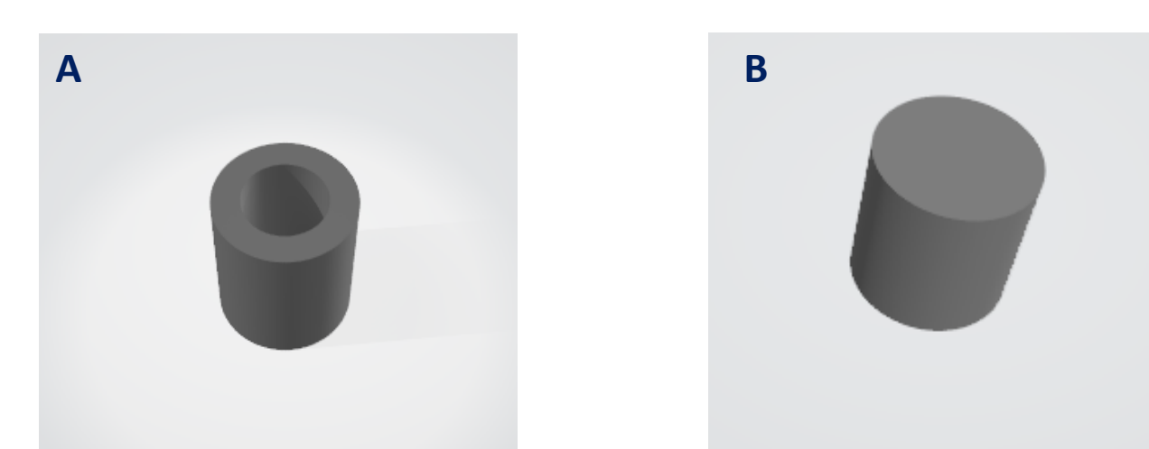
Figure 4. Models of pieces projected with SolidWorks A) Hollow cylinder; B) Full cylinder.
