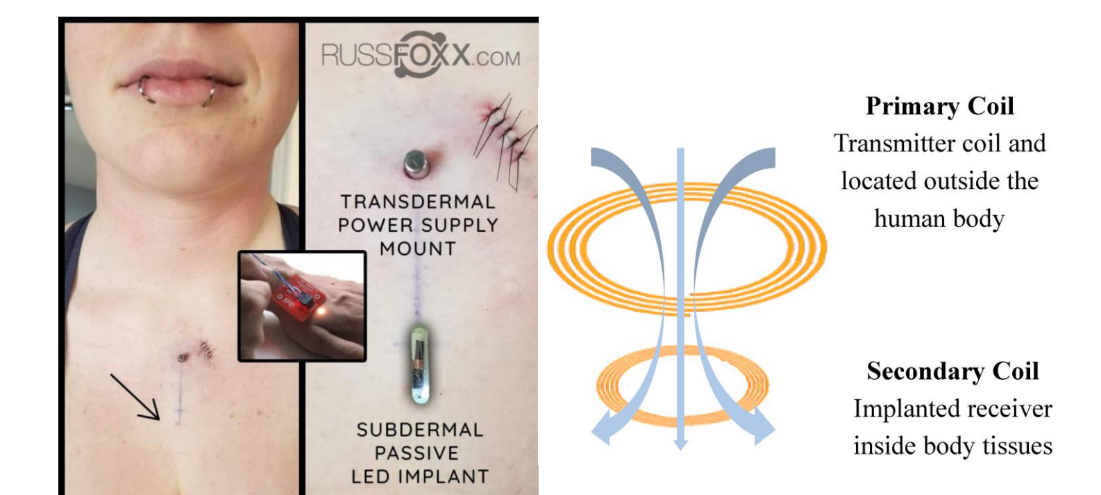
Figure 6: Previous efforts in transdermal power compared to inductive coupling
