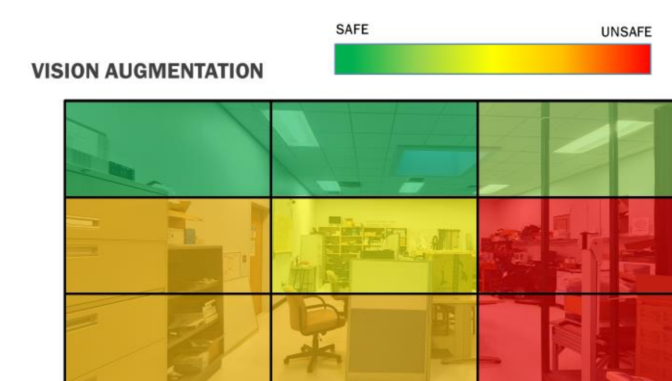
Figure 3: Mockup of future LIDAR grid design
