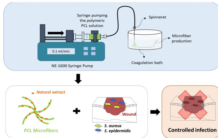
**Figure 1.** Schematic representation of the production of PCL microfibers loaded with natural extracts and antimicrobial action against *Staphylococcus aureus* (*S. aureus*) and *S. epidermidis* bacteria.
