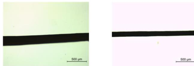
**Figure 2.** Example of the morphology of microfibers unloaded (left) and loaded (right) with thymol, captured at 5× magnification using a brightfield microscope (scale bar = 500 μm).
