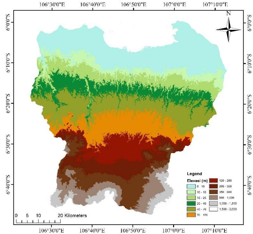
The topography data is derived from the Digital Elevation Model (DEM) obtained from the Shuttle Radar Topography Mission (SRTM). The data was open-source data provided by the United States Geological Survey (USGS). For the SRTM, the vertical accuracy is 16 m for 90% confidence level [45].
