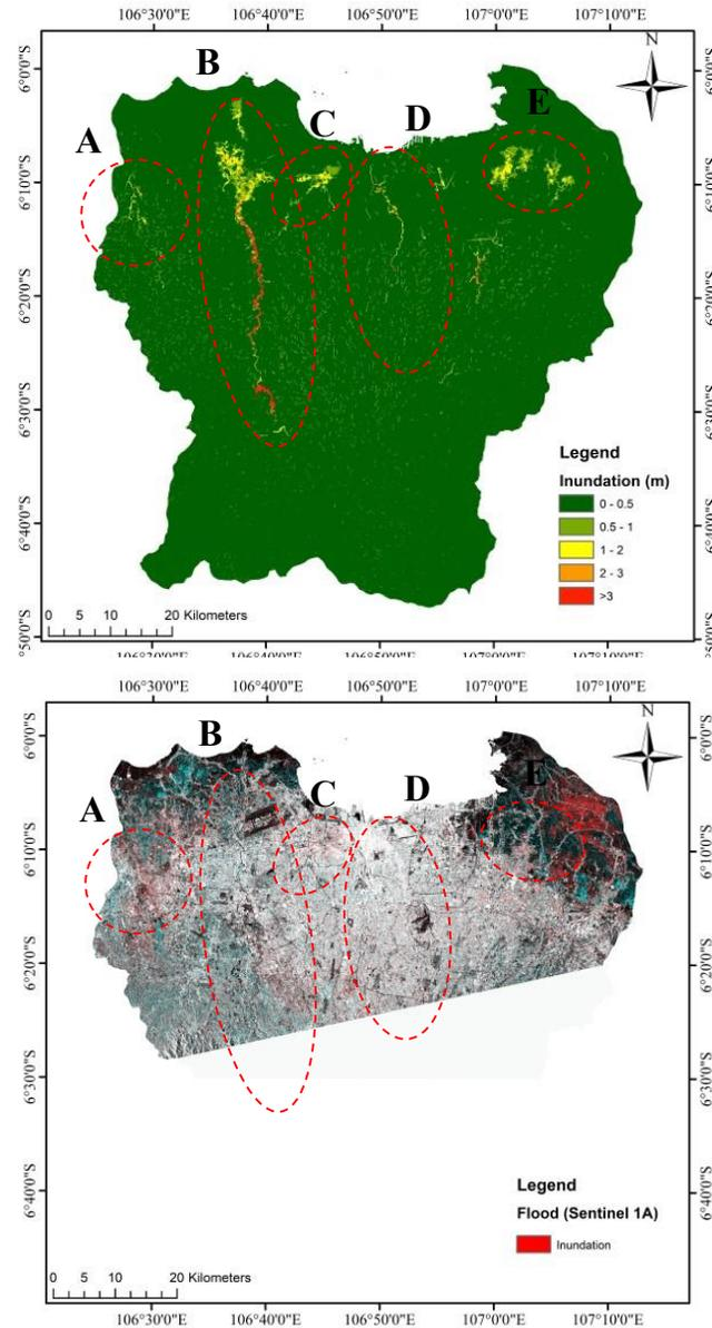
**Figure 7** Rapid Assessment of Jakarta Flood Inundation: (a) simulated 1<sup>st</sup> January flood inundation (b) flood inundation of sentinel 1A acquired on January 2<sup>nd</sup>, 2020
